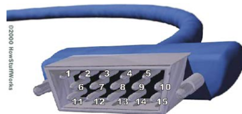
Fig. 1. Pinout information for a standard Male VGA Connector
