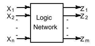
No feedback among inputs and outputs. Outputs are a function of the inputs only.
