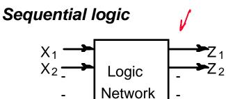
Network implemented from logic gates. The presence of feedback distinguishes between *sequential* and *combinational* networks.
