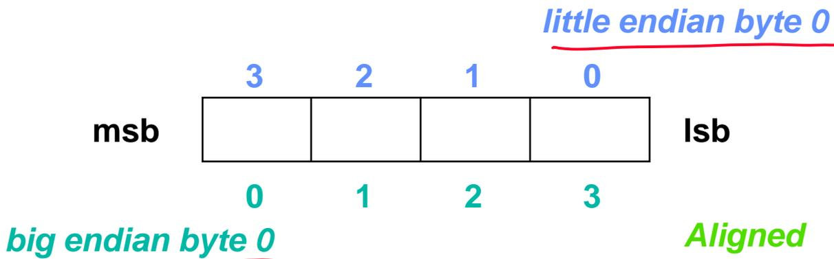
**Alignment: require that objects fall on address that is multiple of their size.**
