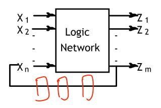
Network implemented from logic gates. The presence of feedback distinguishes between *sequential* and *combinational* networks.
