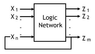
Network implemented from logic gates. The presence of feedback distinguishes between *sequential* and *combinational* networks.
